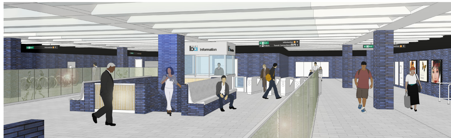
1 Expand Station Capacity Relocate station agent booth and add fare gates to reduce crowding at north end of station
